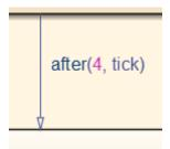
In chart coverage, the after(4, tick) transition represents two conditions: the occurrence of tick and the time delay after(4, tick). Since the temporal event tick is never false, the first condition is not satisfiable, and you cannot record 100% condition and MC/DC coverage for the transition after(4, tick).
