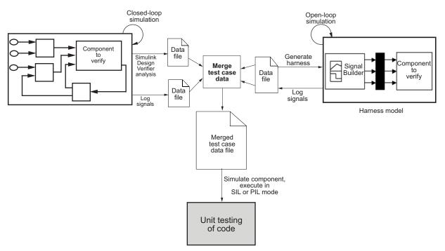
This graphic illustrates the two approaches for component verification, described in "Component Verification" on page 11-2:
