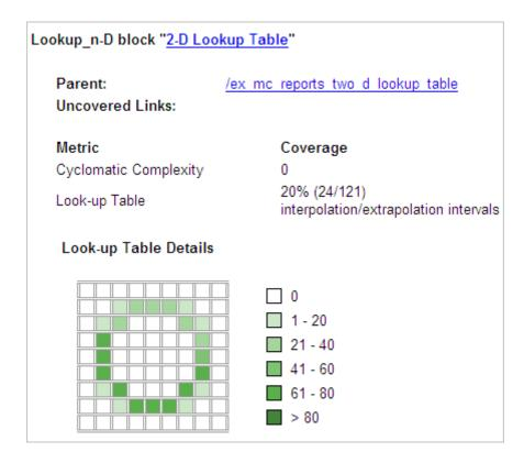
The report contains a two-dimensional table representing the elements of the lookup table. The element indices are represented by the cell border grid lines, which number 10 in each dimension. Areas where the lookup table interpolates between table values are represented by the cell areas. Areas of extrapolation left of element 1 and right of element 10 are represented by cells at the edge of the table, which have no outside border.
