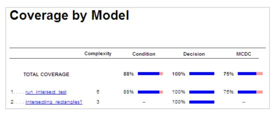
The model coverage report for run\_intersect\_test.m reports the same coverage data as if the functions were stored in the MATLAB Function block.
