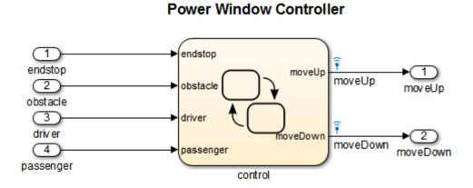
The referenced model contains a Stateflow chart control, which implements the logic for the power window controller.
