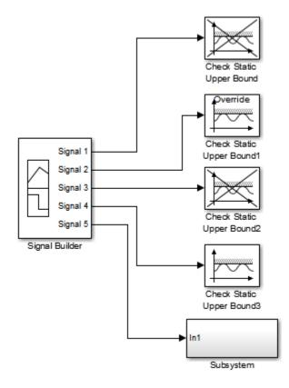
Because you enabled the Check Static Upper Bound1 block in the current group, an **Override** label is applied to the block and it is no longer crossed out.
