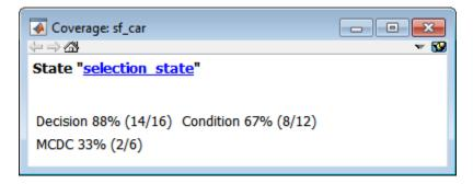
When you click a highlighted Stateflow object, the summarized coverage for that object appears in the Coverage Display Window. Clicking the hyperlink opens the section of the coverage report for this object.
