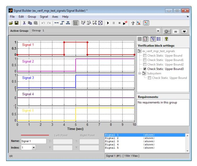
The **Verification block settings** pane lists all Model Verification blocks in the model, grouped by subsystem. If you right-click in this pane, you can select on of three options for viewing Model Verification blocks in this window:
