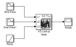
Both the x and y table axes have the indices 1, 2,..., 10. The z axis has the indices 10, 20,..., 50. Lookup table values are accessed with x and y indices that the two Sine Wave blocks generated, in the preceding example, and a z index that a Ramp block generates.
