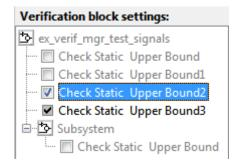
The Check Static Upper Bound2 block is no longer crossed out, indicating that the block is enabled for the current group. Check Static Upper Bound1, however, is crossed out because it is enabled in a different group.
