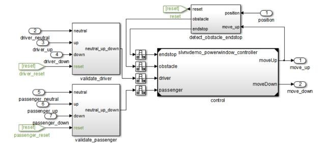
The Model block references the slvnvdemo\_powerwindow\_controller model.
