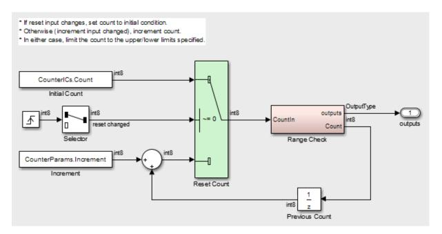
Note the following about the coverage for the Range Check subsystem in this example:
