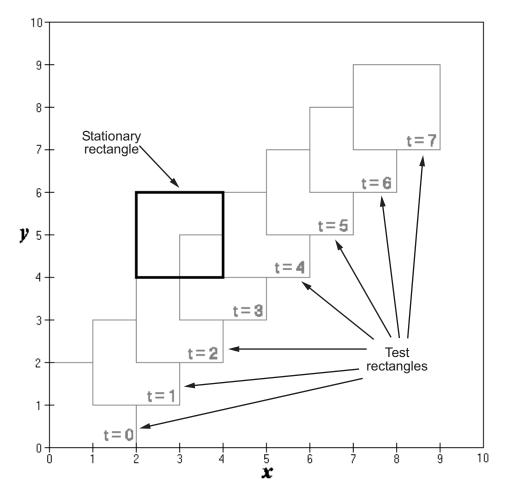
The fixed rectangle is shown in bold with a lower-left origin of (2,4) and a width and height of 2. At time t = 0, the first test rectangle has an origin of (0,0) and a width and height of 2. For each succeeding sample, the origin of the test rectangle increments by (1,1). The rectangles at sample times t = 2, 3, and 4 intersect with the test rectangle.
