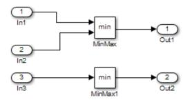
If you set **Force block reduction off**, the report contains no coverage data for this block because the minimum input to the MinMax1 block is always 1.
