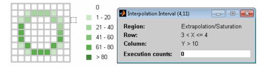
A bold grid line indicates that at least one block input equal to its exact index value occurred during the simulation. Click the border to display the exact number of hits for that index value.
