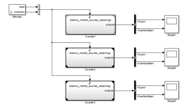
This model contains three Model blocks that reference the sldemo\_mdlref\_counter\_datamngt example model. The corners of each Model block indicate the value of their Simulation mode parameter:
